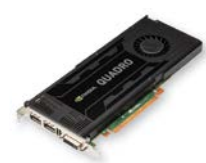
NVIDIA Quadro K4000 Graphics Card 2GB GDDR5 video memory, 256 CUDA cores, one Dual Link DVI-I and two DisplayPort outputs
