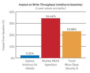
**Note**: A nested 72.4GB file set was used for read transactions. Client load emulated by Load DynamiX TDE 3.2, requesting approximately 9:1 read/write transactions. Test run for a period of 1 hour. Lower impact from baseline is better. Baseline read throughput 43.77MB/s, write throughput, 4.9MB/s
